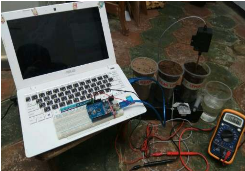
Gambar 9. Perangkat pengujian berupa sensor Soil Moisture Model Stick, analog moisture meter, AVO meter digital, arduino, laptop, kabel data USB, tanah sampel
